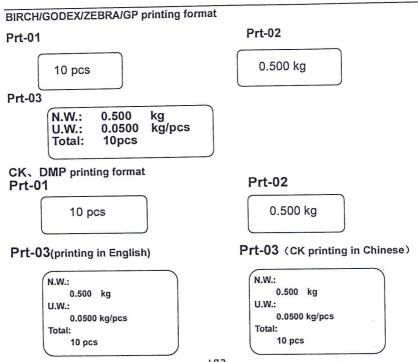
When the window of unit weight shows  $[\Pi]$ , the printing format of accumulation display
